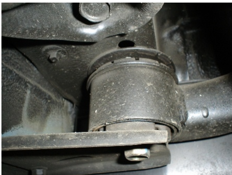
Fig 1. Rear Subframe mount - Original
