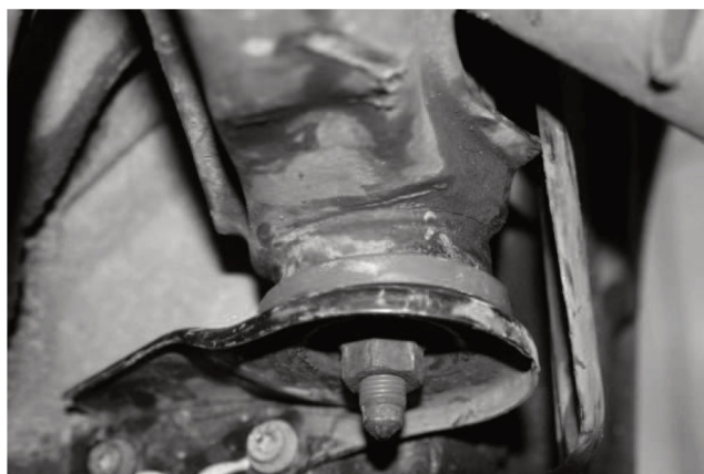
Figure 1 - The assembled rear beam to chassis mount
