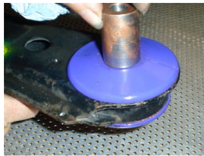
Apply Supplied Lubricant To Sleeve & Push In
