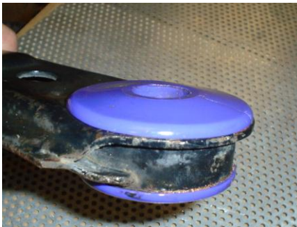
Bush Correctly Installed Into Arm
