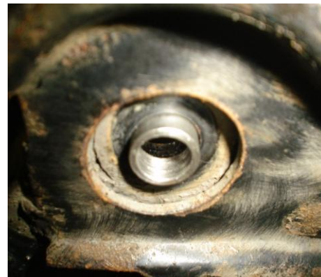
Locate Small Sleeves Into Both Sides Of Bolt Hole
